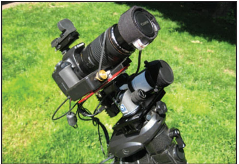
**Image 1 - The author's heliFocus-equipped Canon USM 75-300 lens is shown mounted together with a mini guide scope on his Celestron CG-5GT mount. The versatile bracket included with each heliFocus unit makes it very easy to create a mounting solution for a wide range of equipment configurations.**
